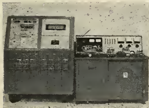
COMPLETELY solid-state and modularly constructed is Stromberg-Carlson's SCATE, a typical advanced automatic check-out system. A survey of this rapidly growing market starts on p. 53.
