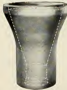
Forging of a Liner -- Exit Cone Missile Material: Unalloyed Arc Cast Molybdenum Diameter of Large Conical End: 10.50" Height: 12.89" Diameter of Small Conical End: 6.75" Weight: 104.5 lbs.
