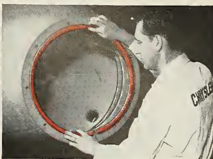
Sealing the nose cone on the Army Redstone is an extrusion of Silastic. Silastic maintains a positive seal despite long periods of storage under load and adverse operating temperatures.
