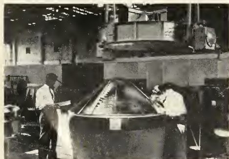
EVERY CONE arriving at the Cape receives a "pit-plotting" inspection for possible shipping damage.
