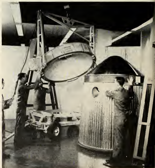
AIR FORCE CREWMEN match a missile nose cone to a simulated Thor instrument section at General Electric's Ordnance Systems.
