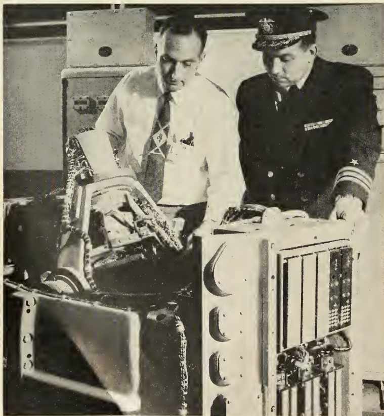
SPERRY MK-3 SINS is ready for the Navy's third and fourth Polaris subs. Foreground, one of three inertial platforms; rear, NAVDAC computer and control cabinets.
