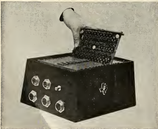
STANDARD PCM system is solid-state throughout, will handle both high- and low-level inputs. Built-in flexibility offers variable bit rate, and trade-off between number of channels and channel information bandwidth.
