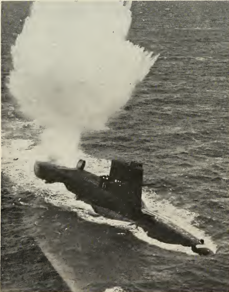
ONE-TON Sabot "slug" is fired from a port missile tube of the George Washington during a drill in Long Island Sound.
