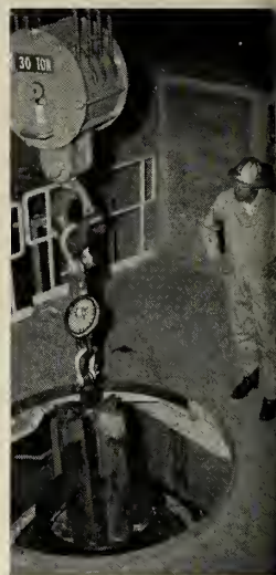
grain-forming core removed from motor; positioning first stage for welding; second stage motor loaded for shipping.
