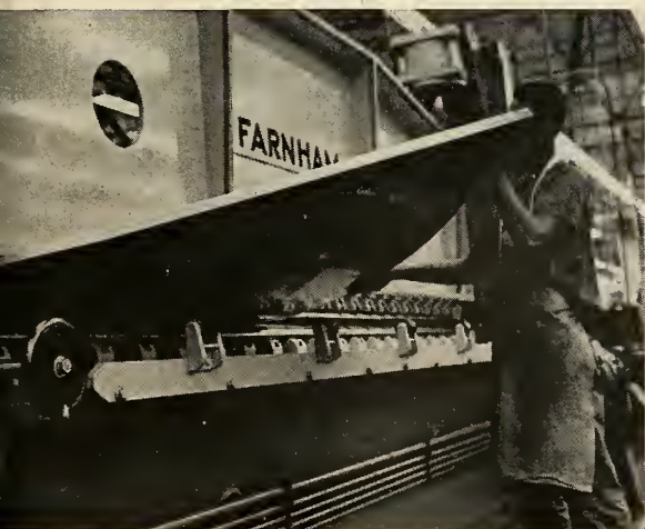
CONICAL SKIRT for Polaris is guided through the giant roll. Lockheed says the technique saves about $50,000 a year.
