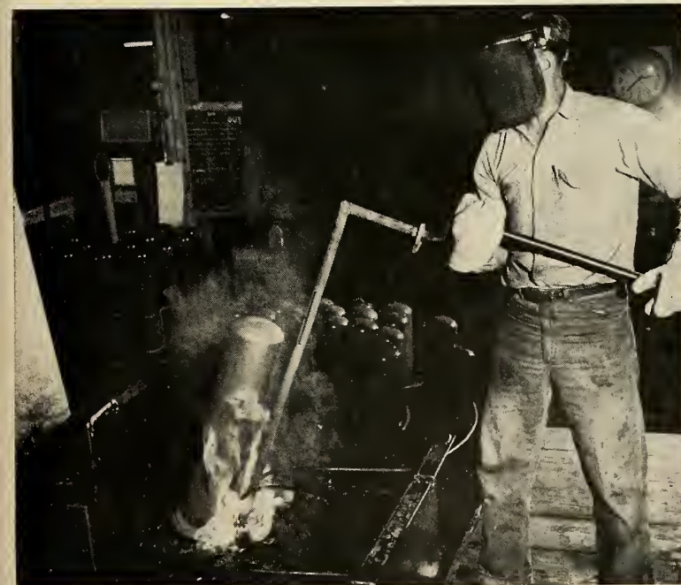
DEEP-DRAWN Falcon motor case being oil-quenched before heat treating operation. missiles and rockets, December 1, 1958
