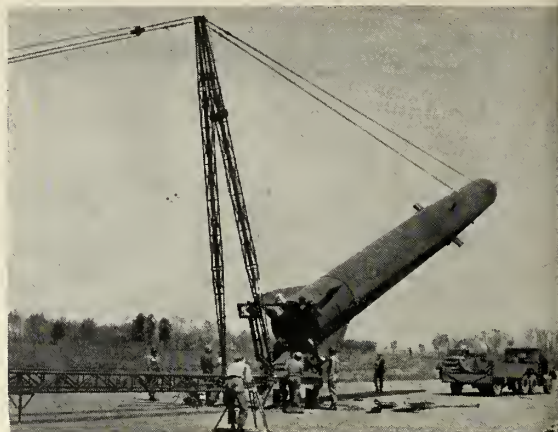
LIGHTWEIGHT GROUND HANDLING EQUIPMENT , used in the Redstone system, will be employed with the Army's new solid-grain Pershing . Army expects to modify these frames, giving simplified mobility and readiness to the Pershing system.
