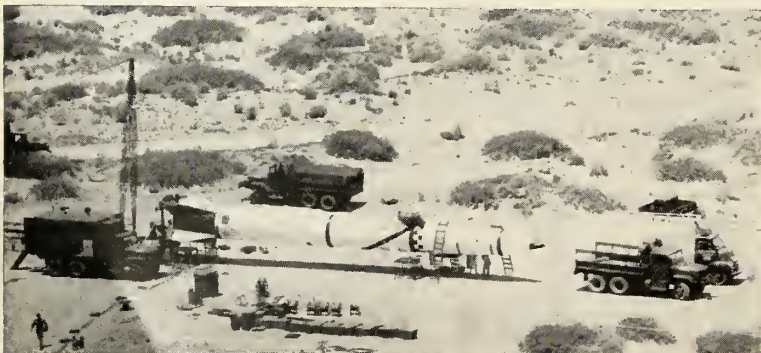
ARTILLERY, 1958—Troops of the 40th Army Field Artillery Group (Redstone) give the giant missile a horizontal checkout before pulling it into vertical position for firing at the White Sands Missile Range. The first simulated firings of Redstone were made with a dummy warhead, though the missile can carry either conventional or atomic warhead.
