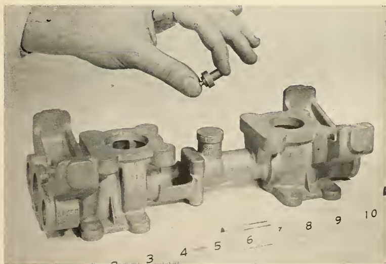
SUCCESSIVE CERAMIC LAYERS are applied by dipping in the refractory slurry and stuccoing. This phase of the operation is slated for mechanization. The final product is shown in comparison to the usual investment casting.
