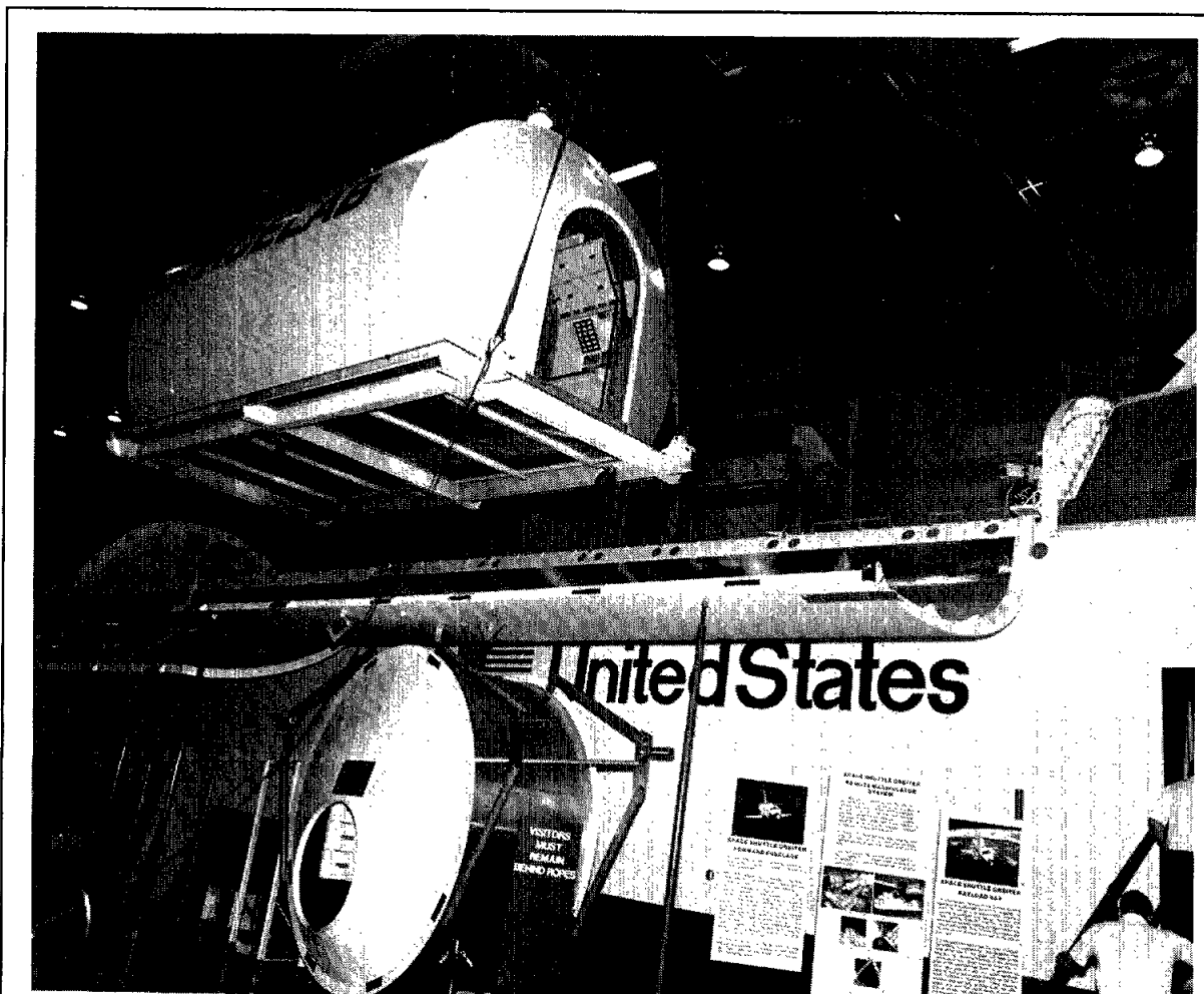
SPACELAB DELIVERY —A full-scale Spacelab mock-up was installed in the payload bay of the Full Fuselage Trainer (FFT) in Bldg. 9A last month. The current FFT configuration, including an airlock adapter interfacing with a transfer tunnel attached to the Spacelab mock-up, allows the crew of STS-40 to step through Spacelab training procedures in preparation for its August flight.
