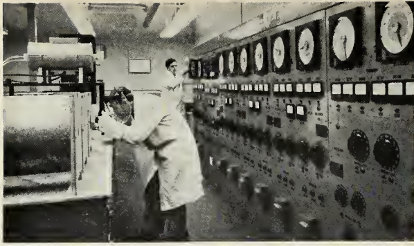
HEAT TREATING furnaces at Nuclear Metals, Inc., where "exotic" metals are investigated for high temperature resistivity.
