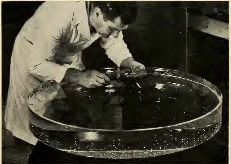
SLATED FOR USE in the Stratoscope II balloon-borne telescope project, this 36-in. fused silica quartz mirror produced by Perkin-Elmer from a Corning blank weighs more than 400 lbs. It is polished to an accuracy of 1/1,000,000 th in.
