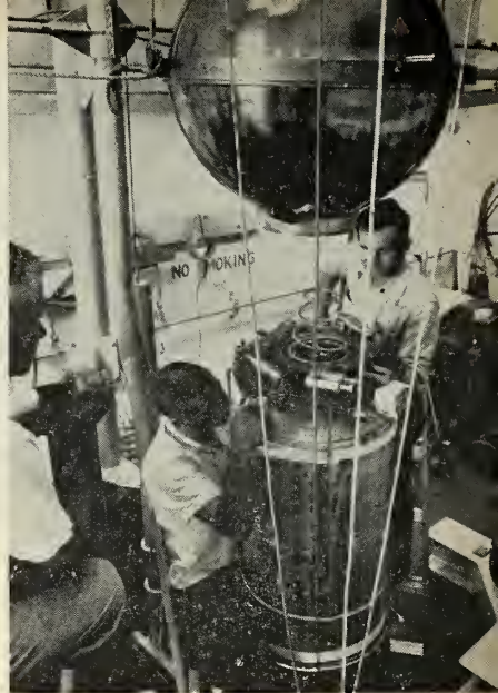
SEPARATION mechanism for Echo sphere shown in Douglas hangar at Cape. Spring throws in away from vehicle's 3rd stage.
