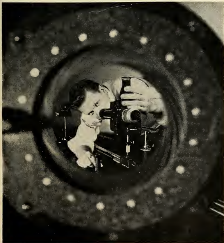
BULOVA ENGINEER checks the optical system of a special camera developed by the company. It is one of several classified photographic units developed for aerial reconnaissance purposes. (The photo was made through a large "master" diaphragm-shutter used in the testing device.)
