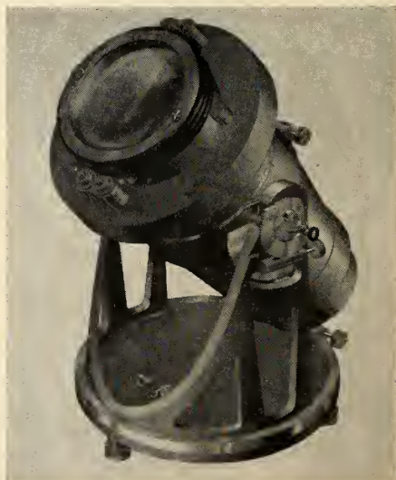
RIGHT: NORTRONICS will develop this 60-millimeter ballistic camera—largest of its type. A recent Air Force contract calls for six of the cameras, which will make use of a new low-type shutter one foot in diameter.
