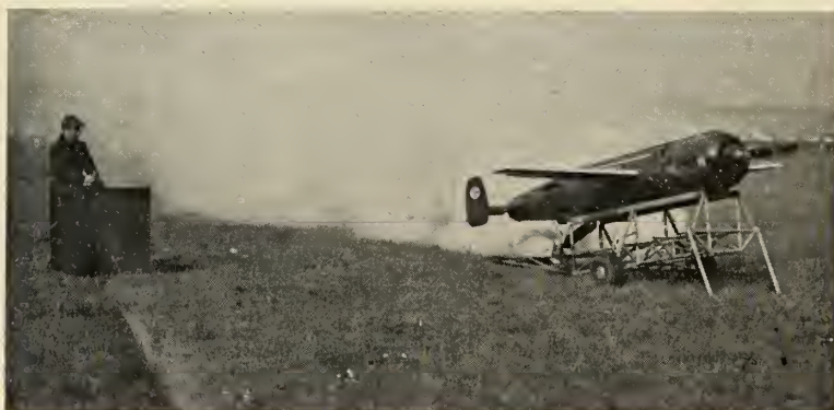
METEOR P.2 "Ricognitore Televisivo Radioguidato" (TV Surveillance Drone) takes off at full RPM of 240-hp four-cylinder radial engine with rocket booster. The drone is under control of VHF 5 modulated tone carrier signal of ground transmitter.
