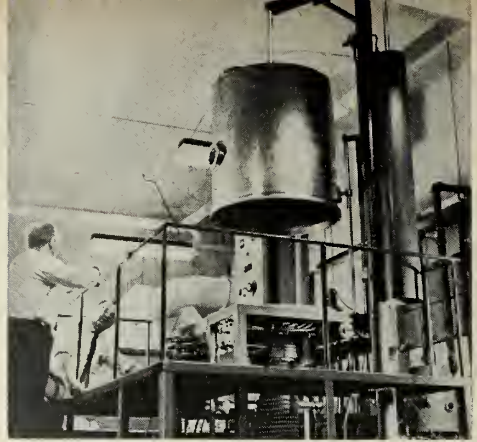
ALUMINUM reflective coating is bonded to plastic replicas in vacuum chambers.
