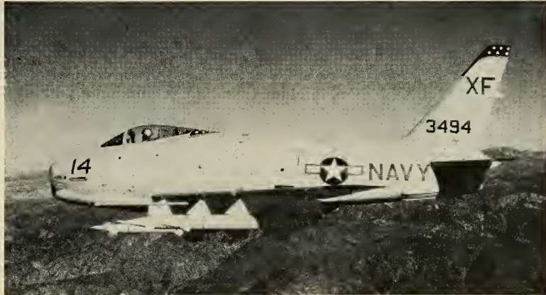
MARTIN's Bullpup tactical air-to-surface missile is one example of the "educated shell" which utilizes integrated electronics.
