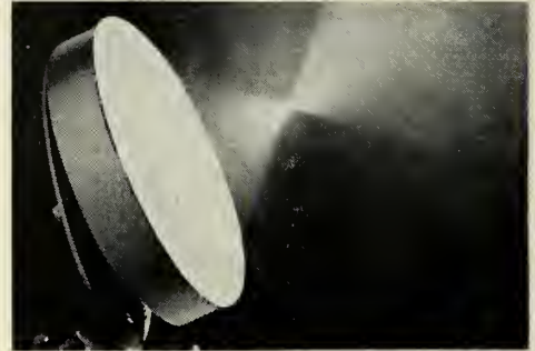
APERTURE of f:0.6 is illustrated by sun rays made visible by smoke.
