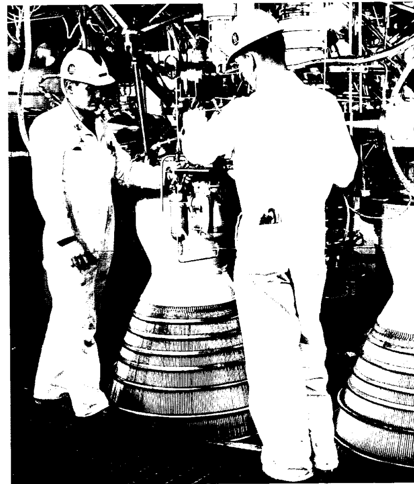
WHITE SUITED—These uniformed Gemini production employees of Aerojet-General Corporation fit engine parts into the powerful liquid engine as the system is readied for delivery to the test area.
