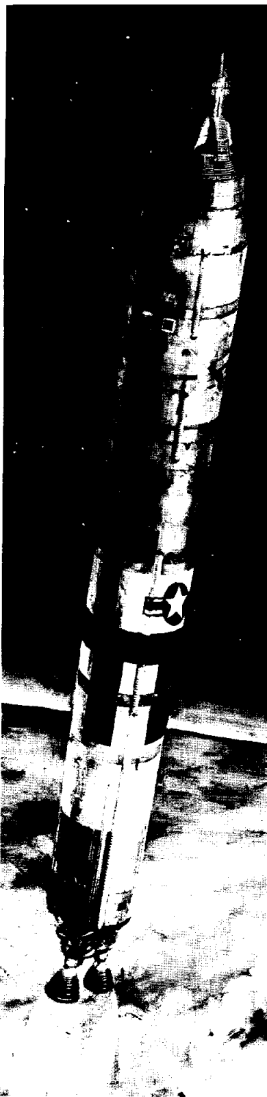
THE GEMINI two-man spacecraft, designed for earth orbital flight, is seen in this artist's concept riding atop its launch vehicle, the Titan II. Both first and second stage liquid rocket engines will be produced by the Liquid Rocket Plant of Aerojet-General Corporation, Sacramento, Calif.
