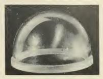
siderably more than a hemisphere, and in aspheric shapes. Physical dimensions are controlled during manufacture to achieve extremely close tolerances. After final grinding and polishing, spherical tolerances are held to millionths of an inch, diameters to ten thousandths, and con-centricity between inner and outer surfaces within ten thousandths.
