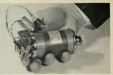
nent of acceleration along its longitudinal axis moves the sensor along this axis for precise electronic measurement.
