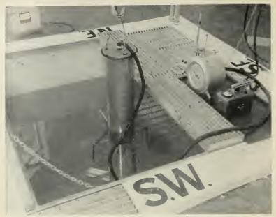
Fig. 4-Production of free radicals by gamma ray bombardment in a cobalt 60 source.
