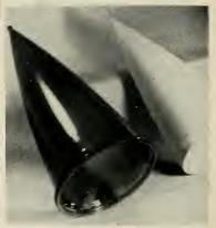
Extensive use of silicone is needed for highspeed missile radomes to overcome the high heat of aerodynamic friction.
