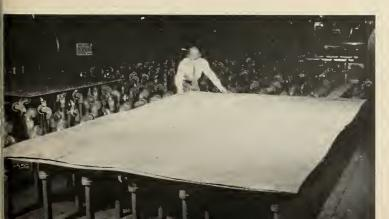
Above—Workman at Homestead Works coating stainless-steel plate with a special separating compound during the assembly of carbon-steel and stainless-steel "sandwich." Use of this compound prevents fusing of the metal plates during the hotrolling process. After rolling, ends and sides of the carbon plates are sheared away; the resulting stainless plates are the widest ever produced on existing mill equipment. Left—Inspector examines finished stainless sheets after rolling.
