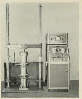
New shock tester—the HYGE-6000—ovoilable with 12", 18", ond 37" long cylinders.
