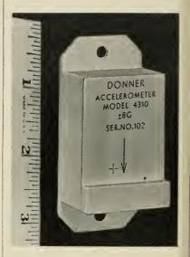
4310 is portable and can be operated from a simple battery power supply providing  $\pm$  15 v at 6 ma. Repeatability is 0.01% of full-scale and linearity is within 0.05% of full-scale. The entire unit weighs only 3.2 oz. When weight and space requirements are even more critical the acceleration pickup portion can be separated from the servo-amplifier part of the instrument and installed in a remote location.
