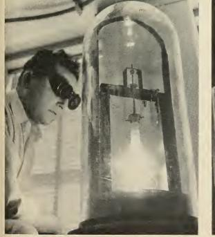
Fig. 4—Testing tensile strength of metals and ceramics.
