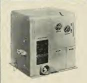
SPECIAL HYDRAULIC POWER UNIT FOR RAIS-ING "NIKE" LAUNCHER OPERATES AT 3000 PSI.
