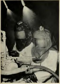
Water is sprayed over protective clothing of engineers to wash away residue as they load fuel into rocket. Transfer line is Aeroquip 610 KEL-F Hose.
