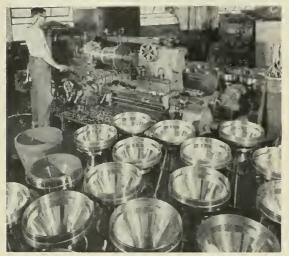
The nozzles are received from the foundry as rough forgings and machined to final shape to maintain the tolerances needed.
