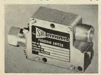
(proof pressure 5000 psig). Actuation to deactuation maximum differential pressure is 250 to 350 psi. Operating temperatures range from  $-40^{\circ}$  to  $+160^{\circ}$ F. Circle No. 227 an Subscriber Service Card.
