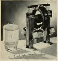
Comparison of size between miniaturized transformer using air as a dielectric and new unit using heavy fluorochemical vapor.
