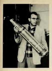
Sealed in polyethelyene to protect it from the elements, EXPLORER I is carried from instrumentation checkout trailer to gantry for mounting on fourth stage of the rocket configuration. Total electronic payload weight was approximately II pounds, total payload 17 pounds.
