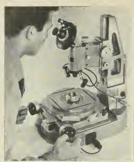
Gaertner Toolmakers' Microscope used to measure typical piece part. Co-ordinate range 4" x 2".
