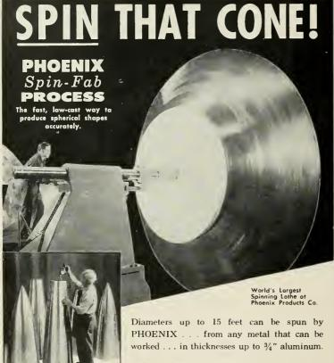
Nose and aft sections, Phoenix fobricated
