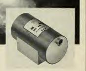
ACCURATE, CONSISTENTLY RELIABLE AC output, proportional to linear acceleration, is provided by this new Giannia accelerometer. Available in ranges from  $\pm 1$  g to  $\pm 20$  g, the instrument has a full scale output of 6 volts which may be fed directly into a relatively low impedance with little or no phase shift.
