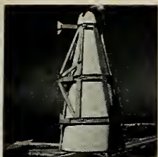
COVER: An Air Force experimental Atlas ICBM nose cone, which on July 21 became the largest re-entry vehicle recovered after intercontinental flight. Built by GE.
