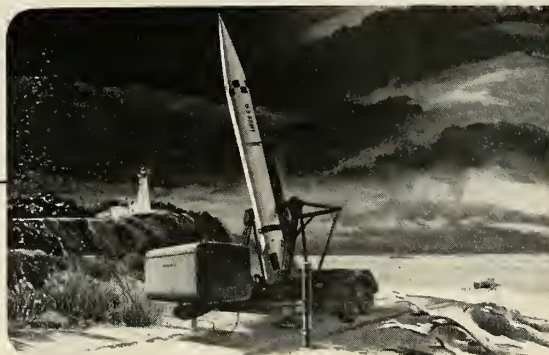
THE SERGEANT... A second-generation solid propellant missile developed by JPL for the U.S. Army. The SERGEANT is now being readied for production.
