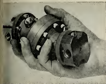
VICKERS hot-gas motorpump. Unit shown, smallest in series, is capable of 1.9 hp and weighs only 2.5 pounds.
