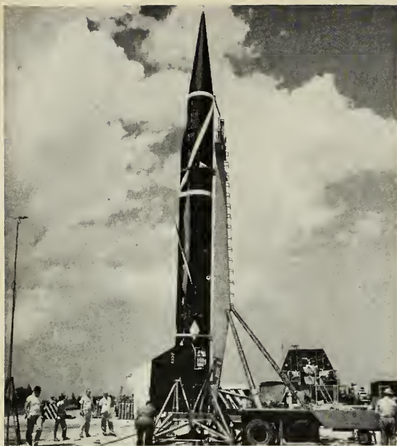
LIGHTWEIGHT launch pad is attached to missile and rests on ground. Transporter moves away from missile for firing.
