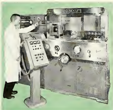
MODEL HCS-59 ELECTROLYTIC CAVITY-SINKER. APPLIES SAME BASIC ELECTROLYTIC PRINCIPLE TO THE SINKING OF IRREGULAR HOLES AND SHAPES FOLLOWING THE CONTOUR OF THE ELECTRODE MADE FOR THE PURPOSE THE ELECTRODE IS SIMPLY PLUNGED LINEARLY INTO THE WORK MATERIAL.
