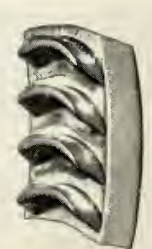
ELECTROLYTIC TREPANNING. DESIRED FORM EXTENDS INTO INTERIOR OF SHAPED ELECTRODE. NOTE HIGH FINISH ON BLADE FORM.
