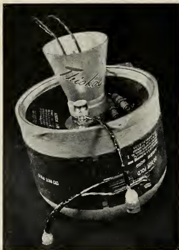
THIOKOL TE 316 Retrograde Rocket Engine for Mercury manned capsule, showing igniter leads, pressure-sensing switch and heater blankets.
