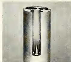
HEXAGONAL HOLE 1" DEEP, 1/4" ACROSS FLATS, IN UDIMET 700. NOTE STRAIGHTNESS AND SHARPNESS OF WALLS WHERE ELECTRODE BROKE THROUGH. CONICAL TIP IN BOTTOM OF BLIND HOLE CAN BE ELIMINATED. INTERIOR-COATED ELECTRODE USED FOR ROUND HOLES IN BACKGROUND.
