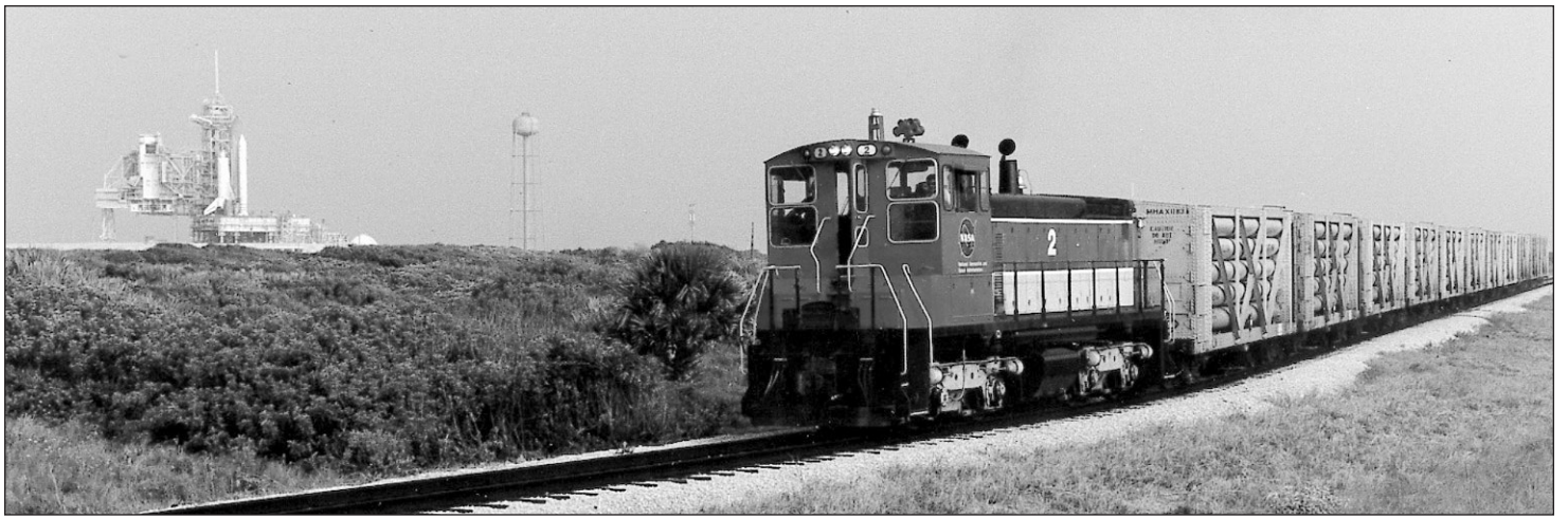
KSC Railroad Engine #2, a GM EMD MP15, hauls a set of 10 Gaseous Helium Transport Cars east of Launch Pad 39A on May 19, 1998, where the Space Shuttle Discovery awaits liftoff for its STS-91 mission.
