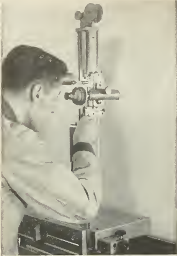
M1238-1818—Range 18" x 18", working distance 9" to infinity. Reads to 0.001" up to 24" working distance. Protractor ocular reads to 3 minutes of arc. Image is erect.
