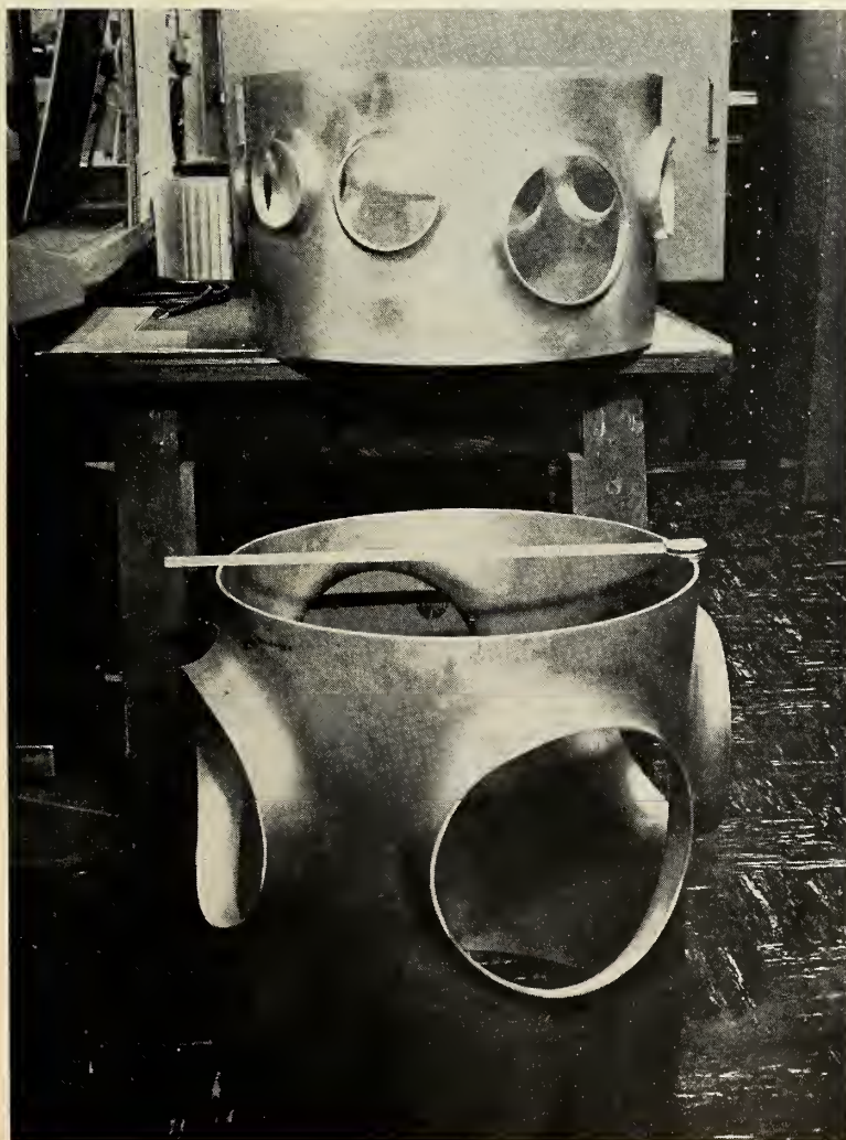
SATURN LOX manifolds shown after explosive flaring of outlet holes by Olin Mathieson in a process invented by research engineer Earl A. Hasemeyer.
