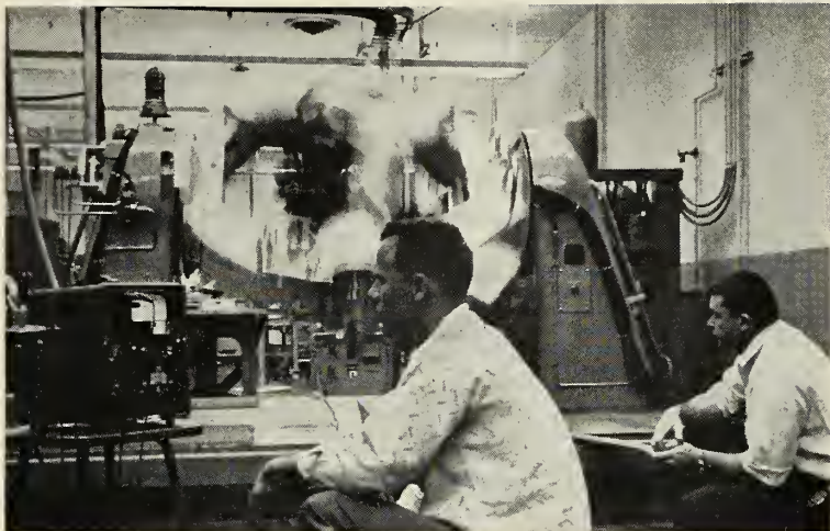
MOTION OF THREE-AXIS flight simulator table is evident as gimbal rates are checked out by technicians at Lockheed's Missile and Space Division.
