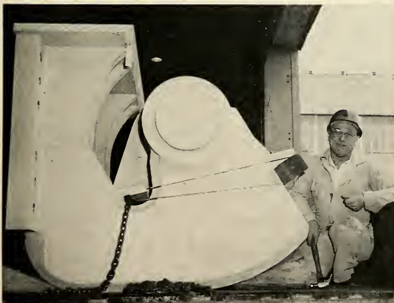
MAMMOTH 600-TON hinges will be used to open the doors of underground Titan launch silos. Nearly five feet high, this is one of a set flame-cut and machined by Lukens Steel Co. for American Machine & Foundry Co.
