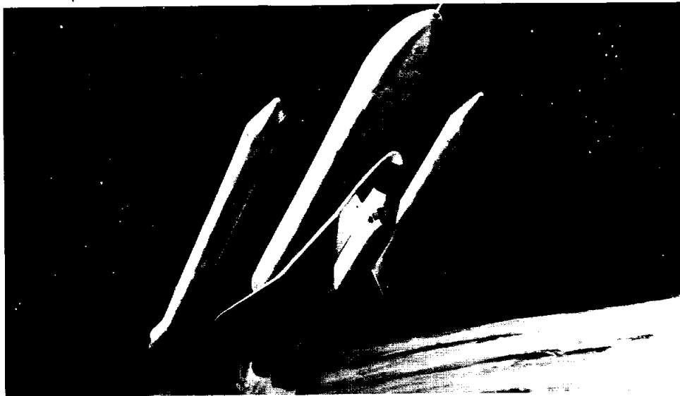
Solid rocket boosters (SRB's) separate from the shuttle in this artists conception. Marshall Space Flight Center completed six drop tests with the booster Sept. 12, confirming their reusability.
