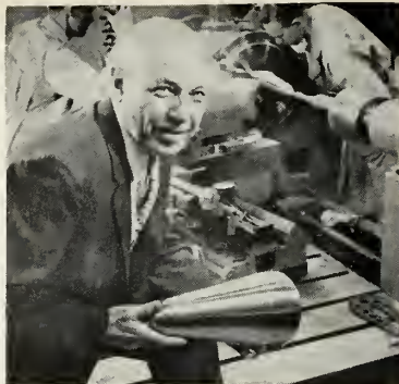
NOSE CONE for Explorer is product of Cincinnati Testing Labs. "Floturning" is the process.
