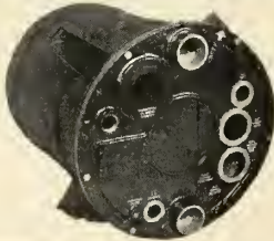
Electronic guidance equipment mounted to both sides of UAP cold plate, contained in UAP pressurized case... for control of air-to-air missile.
