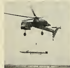
NEW MOBILITY for Honest John is demonstrated by the Sikorsky S-60 crane helicopter which can carry a six-ton load.
