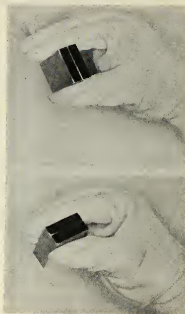
UNSYMMETRICAL thermal effects were produced when gage blocks were gripped as in the top illustration. NBS experts found that this was eliminated when the non-gaging edges were facing the palm as in the lower photo.
