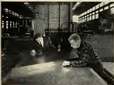
TOOLING PLATE, extra flat, is annealed to eliminate residual stresses.
