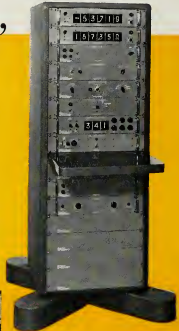
Multi-purpose digital system for measuring a variety of transistor parameters while the transistors are being subjected to environmental testing.
