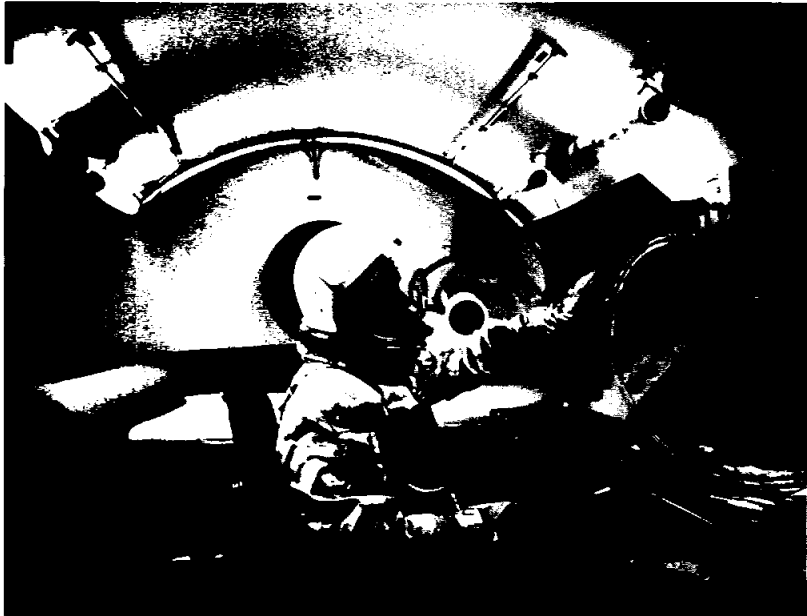
GEMINI SUIT TEST —Hoyt Maples, test subject for the four-day Gemini suit comfort test, is shown operating the task panel in the eight-foot diameter pressure chamber in Building 7 here at the Center.
