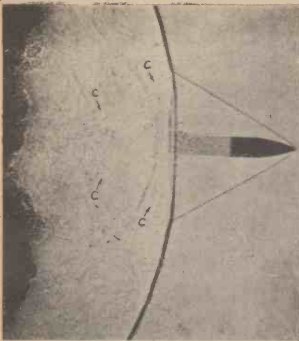
Photograph of a bullet in flight, showing compression waves. The bullet is 11 in. from the gun muzzle—a .30 calibre Springfield rifle was used in the experiment—and, travelling in the region of 3,000 ft. per second, has outdistanced the discharge waves. Note the deflection of the conical bow waves in the explosion wave area, indicated by the arrows "C"; also the stray powder particles which have created compression waves on their own account. (Taken by P. P. Quayle, of the American Bureau of Standards). Courtesy of Kodak, Ltd.
