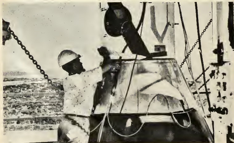
FINAL ADJUSTMENTS are completed on mated first and second stages of missile.
