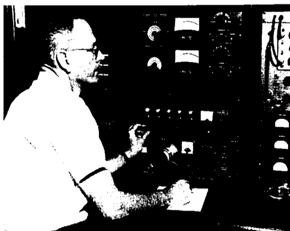
ARTHUR C. CHAPMAN , electronic development technician, of the Structures and Mechanics Division, Experimental Dynamics Section, operates a Sine Console for a vibration system.
