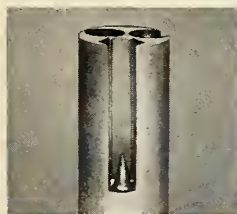
HEXAGONAL HOLE 1" DEEP, 1/4" ACROSS FLATS, IN UDIMET 700. NOTE STRAIGHTNESS AND SHARPNESS OF WALLS WHERE ELECTRODE BROKE THROUGH. CONICAL TIP IN BOTTOM OF BLIND HOLE CAN BE ELIMINATED. INTERIOR-COATED ELECTRODE USED FOR ROUND HOLES IN BACKGROUND.
