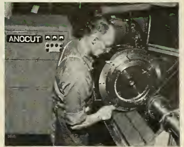
MOUNTING STATOR RING FOR ELECTROLYTIC MACHINING OF VANE TIPS TO ACHIEVE PRECISE CONCENTRICITY AND SIZE. OPERATION IS FAST AND ELIMINATES DEBURRING, SAVING LABOR COSTS AND REDUCING SCRAP.
