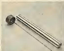
SEVEN INCH LONG, .078" DIAMETER HOLE ELECTROLYTICALLY "DRILLED" IN UDIMET 700. ROD HAS BEEN SURFACE GROUND TO EXAMINE STRAIGHTNESS OF HOLE. NO WEAR ON ELECTRODE.
