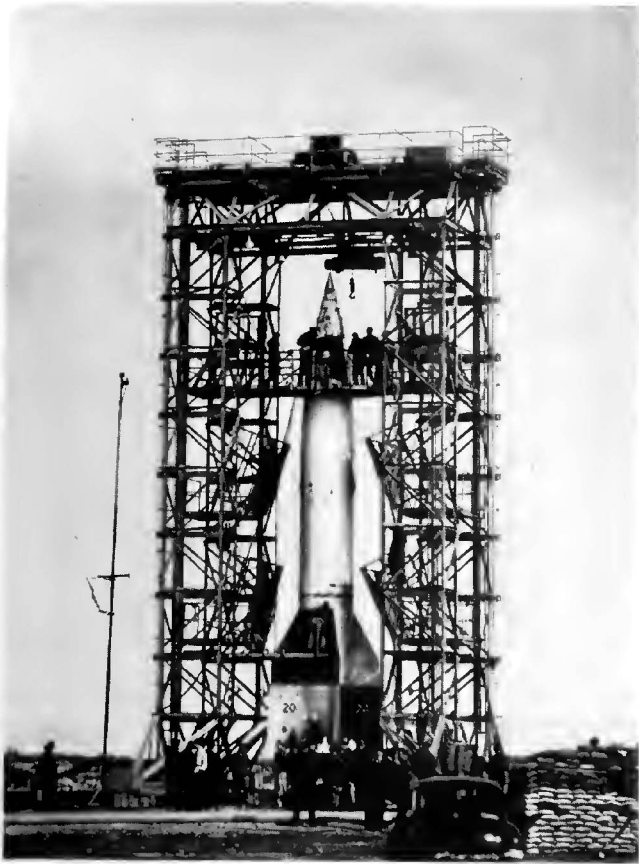
Fig. 5. Final instruments are placed in V-2 by technicians prior to flight into ionosphere.
