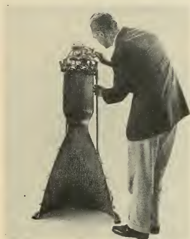
ENGINEER checks valves on cutaway, full-size model of NASA's 6000-pound thrust Vega rocket vehicle.
