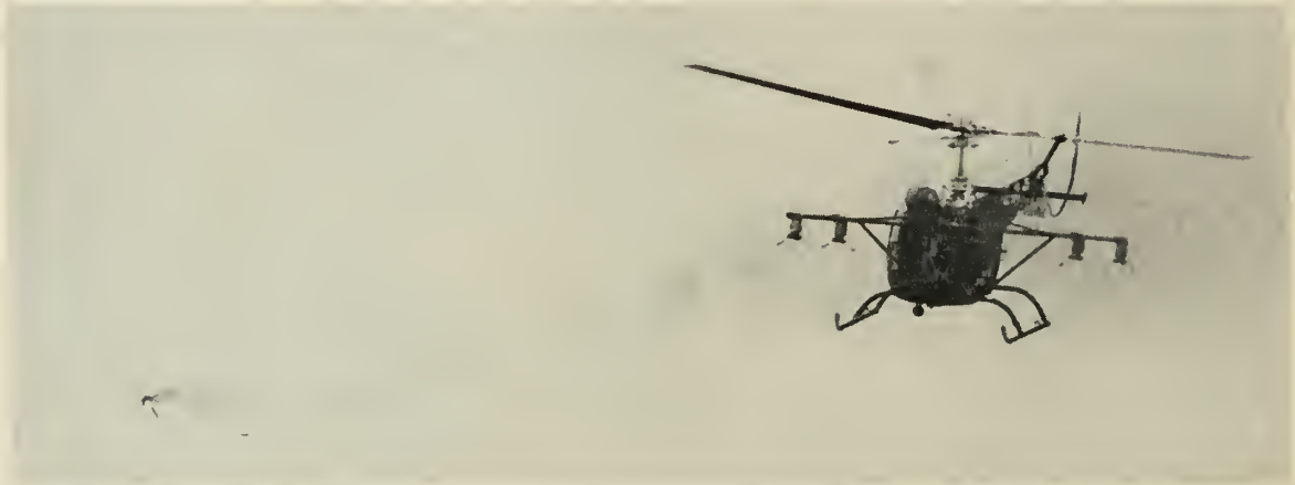
WIRE-GUIDED SS-10 (far left) flashes from Bell H-13. Explosive bolts remove launcher and wires after firing.
