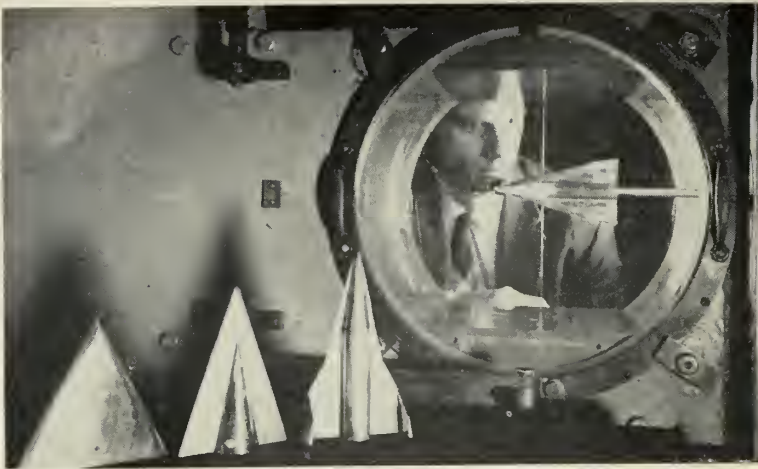
AT LANGLEY Research Center's 11-inch hypersonic wind tunnel, models used include basic flow and heat transfer wing, wing-body combination and re-entry vehicles.
