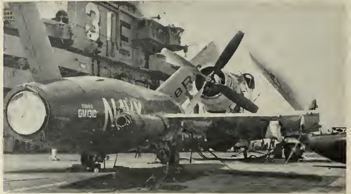
ENERGY FROM aircraft search radar (in rear) is beamed at Regulus I missile with booster during the Radllaz program directed and funded by the Navy's Bureau of Ships.
