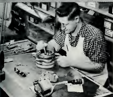
Actuators for jet vanes, air control-surfaces. This rotary actuator is driven by 1 hp d-c servo motor (shown in foreground with cable attached). Both motor and actuator are made by Ford Instrument.
