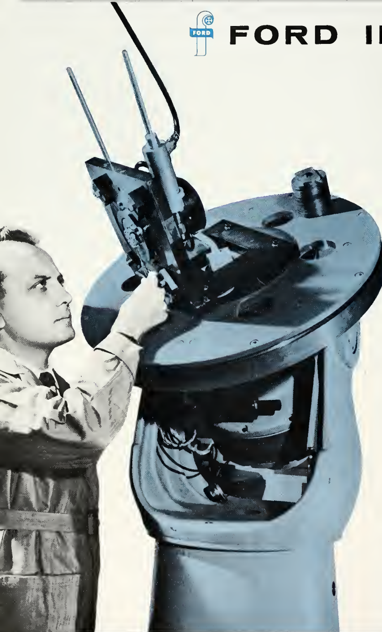
Equatorial test stand, built by Ford Instrument for its own laboratory facilities, is used for conducting basic drift error research. This type of unit can also be built to contractor order.
