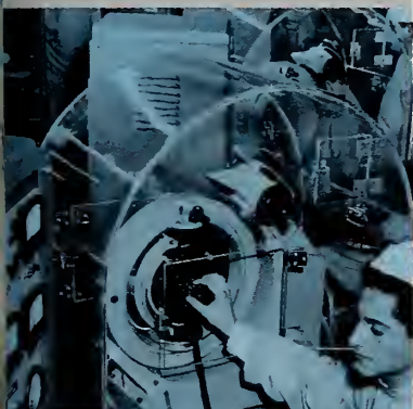
Specialized gyros and accelerometers. Ford Instrument pioneered in the quantity production of air-bearing gyroscopes and accelerometers. Air-bearing gyro here undergoes final test in special Ford-built test equipment.
