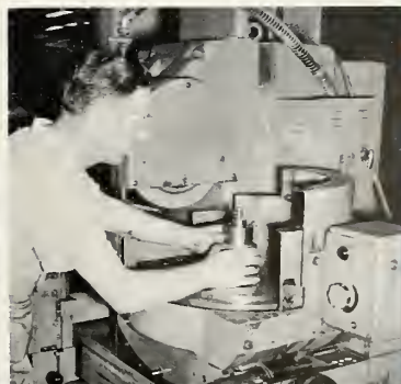
Technician grinds gyro part to a length within 20 millionths of an inch—typical of tolerances being met in missile work at Ford Instrument.
