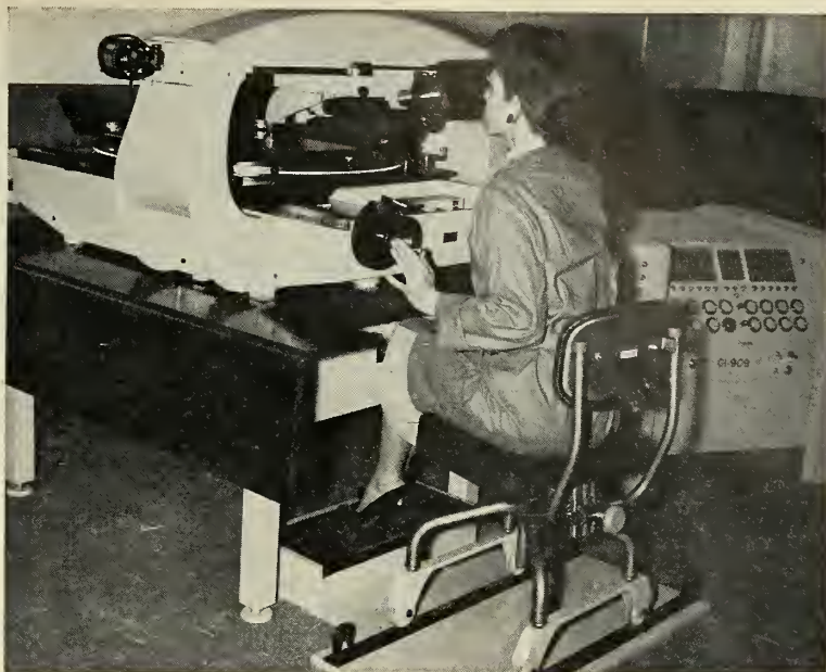
ADDITIONAL INPUT is provided by many optical tracking stations, particularly during early thrust phase of an ICBM. Here, a large-bed Mann comparator permits rapid measuring of film to resolution of 1 micron. Output is fed to Telecorder (right), stored in digital form, then transferred to IBM summary punched cards.
