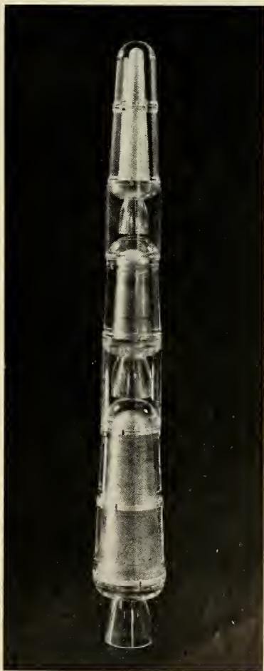
THREE-STAGE ROCKET assembled of conical segments is shown with cases and connecting fairings transparent for demonstration.
