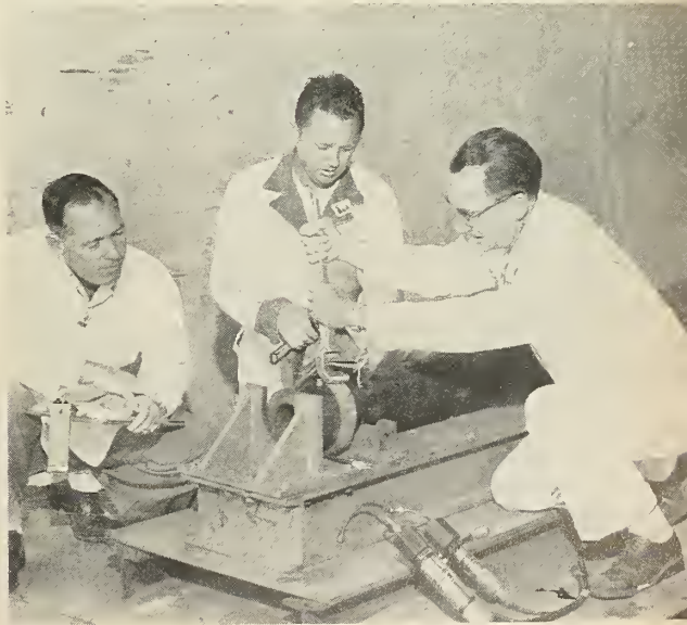
LEFT—Test mechanics lowering a motor into a conditioning box. RIGHT—Final checking of nozzle fit before clamping motor to stand.
