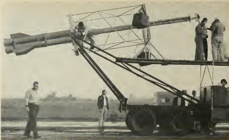
Four-stage Far Side rocket plus its firing platform are mounted on a truck prior to hooking onto 3,750,000 cubic foot General Mills balloon in preparation for June test flight.
