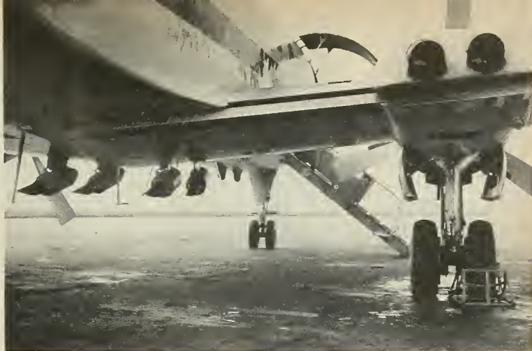
Convair 240 equipped with 15KS-1000-AI standby motors mounted externally and internally.
