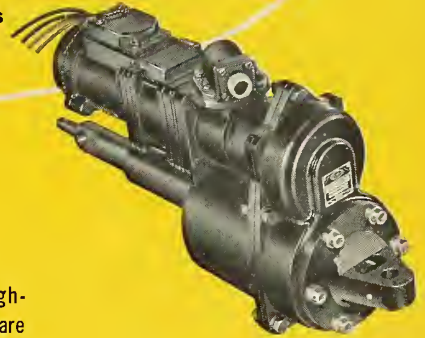
Type: D-818 Leading Edge Flap Actuator; Weight: 20.5 lbs. Normal Operating Load: 6,000 lbs.; Maximum Operating Load: 12,000 lbs. Ultimate Static Load: 24,000 lbs.; Stroke: 3.15"; Rate of Travel: .33" per second; Amperes: 3 amps at 480 cycles on 200 volts at the 6,000 lbs. load. Meets Mil. Specs.: MIL-A-8064 for actuators, MIL-M-7969A for motors.
