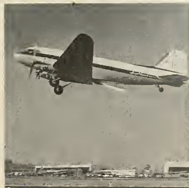
DC-3 is assisted in takeoff with 15KS-1000-AI standby rocket motor. This unit is the only rocket motor that has received CAA certification.
