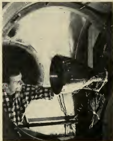
Final instrumentation check-out is made on rocket engine thrust chamber in test section.
