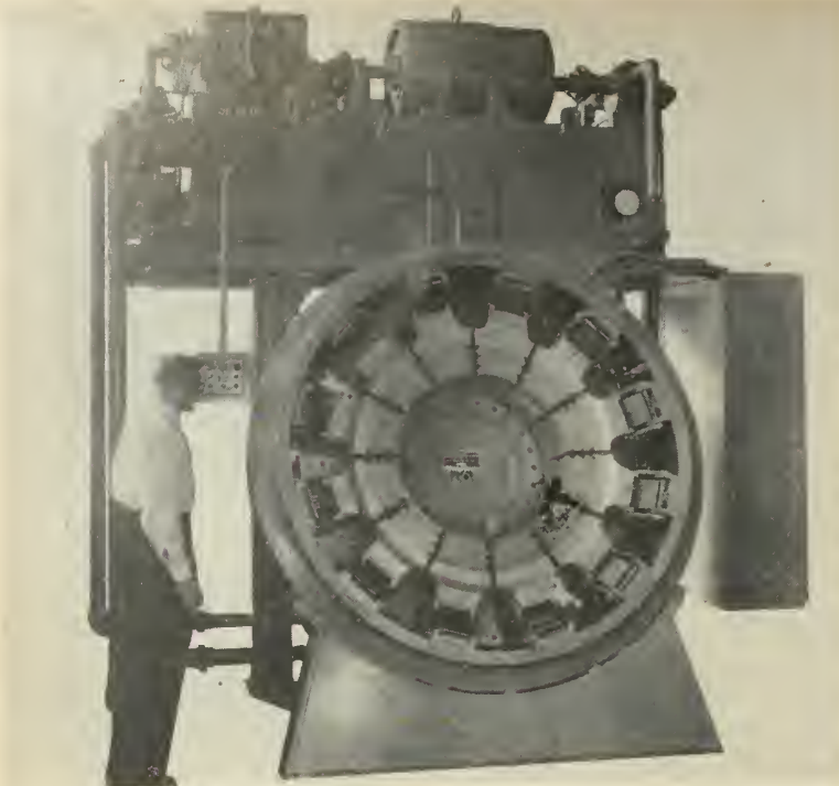
View looking into the 'maw' of a shrinker. Simplicity of operation can be seen in the control box arrangement at left. This shrinker sizes heavy ring sections of stainless steel, aluminum, alloy steel and titanium.
