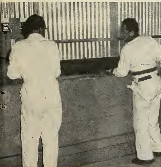
LEFT—Test mechanics lowering a motor into a conditioning box. RIGHT—Final checking of nozzle fit before clamping motor to stand.
