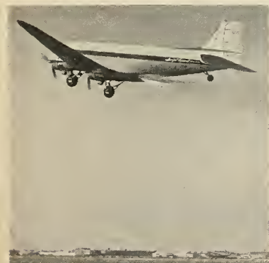
DC-3 is assisted in takeoff with 15KS-1000-AI standby rocket motor. This unit is the only rocket motor that has received CAA certification.
