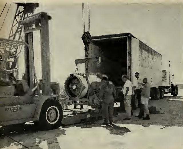
THIRD STAGE is lifted from truck during transport to Cape. Note Blowout ports in forward bulkhead, to terminate thrust.
