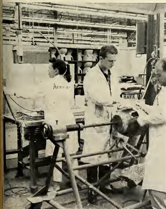
INNER PLASTIC BODIES are cast in form of attached hemispheres (on shelf in background). These are separated, then tops and bottoms cemented together. Hollow shell is then wrapped with tape and covered with metal slugs.
