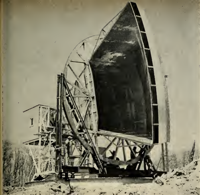
HORN ANTENNA of world's most sensitive radio receiver helped prove principle of passive communications relay by receiving signals from Echo balloon satellite.
