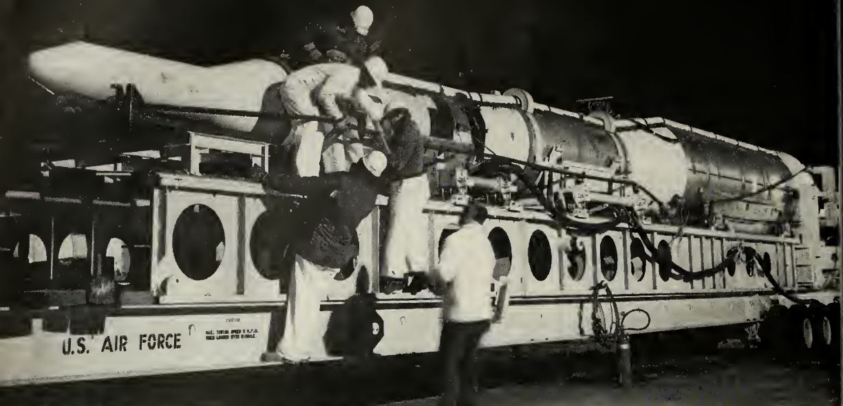
ON EXPERIMENTAL TRAILER, operational configuration Minuteman is readied for silo test shot.
