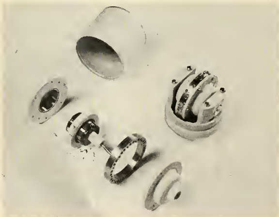
CRITICAL PARTS of first ceramic gyro are made of new gem-hard material diamond-honed to extreme tolerances. Spin-motor, gas-lubricated bearings, and gimbal are all made of the new ceramic. Motor stator is glass-encapsulated.
