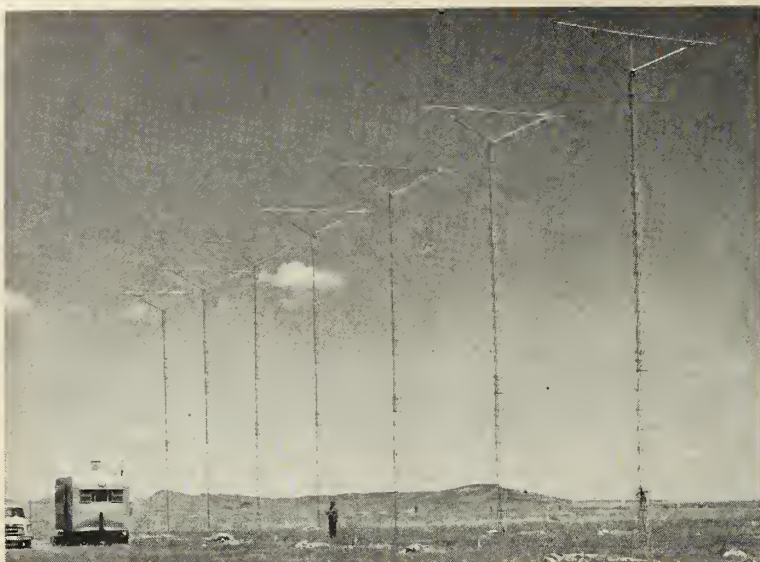
UNIQUE SYSTEM using seven 5-element Yagi antennas in conjunction with an electronic scanning device will be employed soon by NBS to observe ionosphere.
