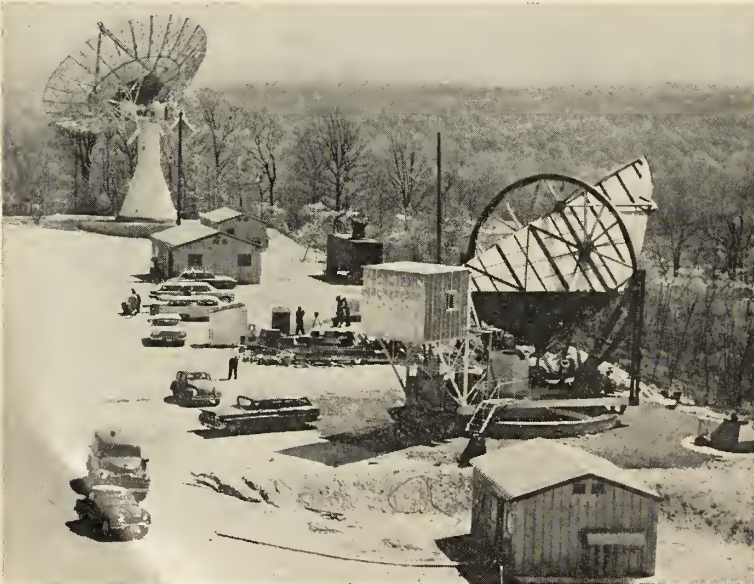
HOLMDEL TRANSMITS signals with 60-ft. parabolic dish antenna. Horn antenna (right) is part of low-noise receiving system. Signals received by horn are amplified by ruby-maser amplifier located in cab at apex of horn.
