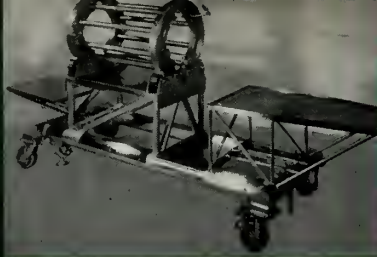
Assembly test stand for transporting and restraining missiles during depot checkout procedure.
