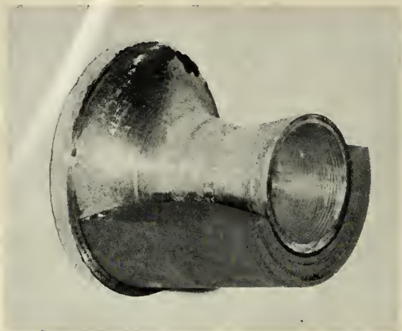
TUNGSTEN ELZ-ZON (nozzle insert) made by vapor deposition process is shown full-scale. High-temperature problems are lessened by housing in loosely fitting graphite blocks.
