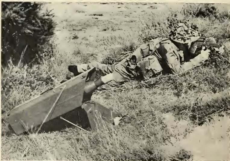
VICKERS VIGILANT has been ordered for trials by the British Army. The wire-guided antitank missile is controlled by hand-held sight-controller.
