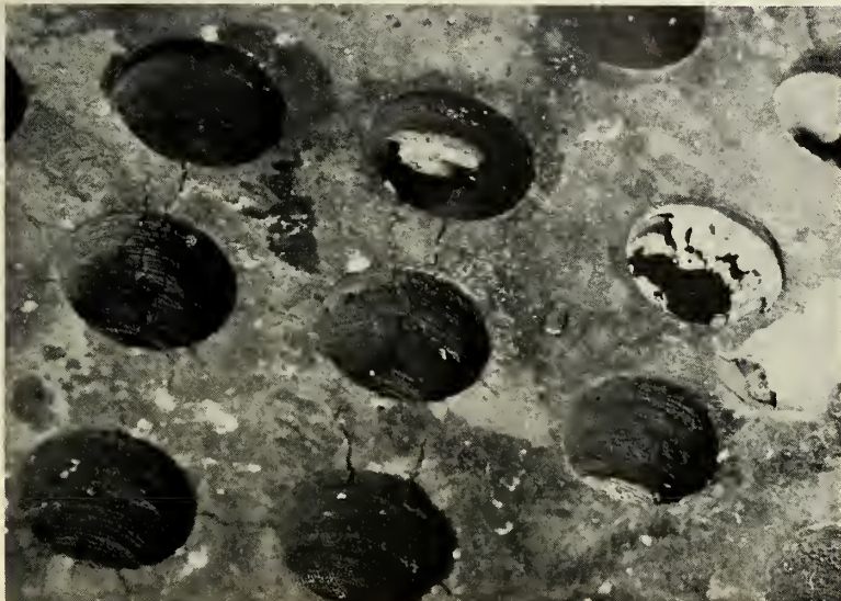
ACCUMULATED OPERATING time of one hour resulted in these cracks in a plate of type 304 stainless steel contained in the lithium hydride system.
