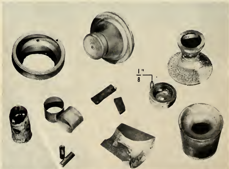
SPECIMENS OF simple and complex forms and coated objects produced at NBS. Note plated rocket nozzle (right bottom) and thick solid-tungsten cap (right center).
