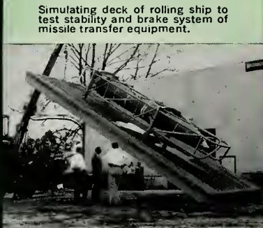
Assembly test stand for transporting and restraining missiles during depot checkout procedure.
