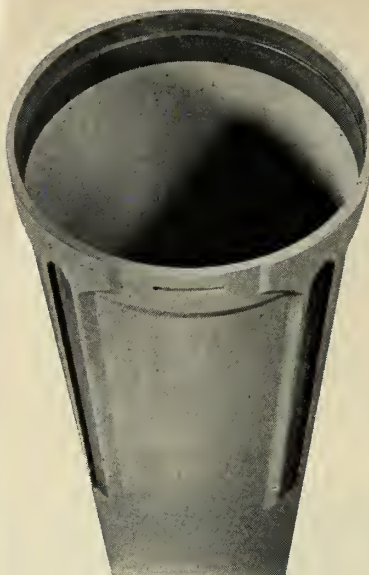
EXPERIMENTAL motor chamber was drawn with integral ribs. This allowed simple, accurate attachment of fins.
