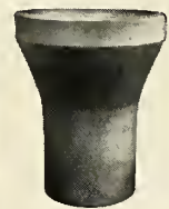
A first stage Polaris Nozzle Liner forged from pure molybdenum.
