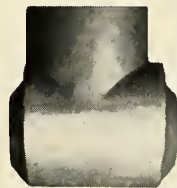
Check Valve for the Hot Loop of Nuclear Propulsion System. These are the largest closed die stainless steel forgings ever produced.
