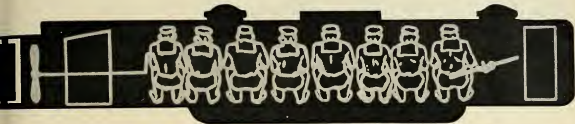
CUTAWAY OF CONFEDERATE SUBMARINE Hunley , first sub to sink a ship in war, shows crew seated at crank shaft used to propel vessel. Hunley sank the USS Housatonic in 1864, but explosion also sank sub and drowned its crew—Navy Photo.
