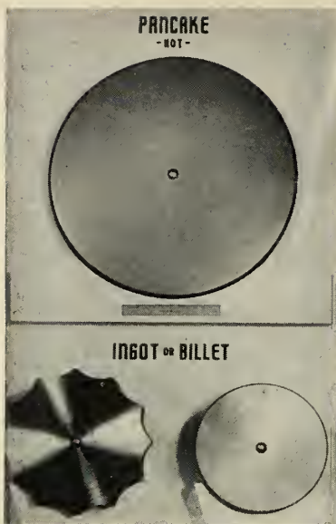
PANCAKE pressed from machined ingot results in formation of radial flow lines ideal for deep drawing.
