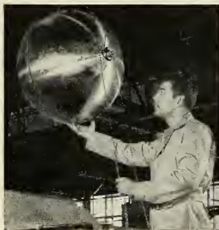
Successful titanium welding techniques have enabled fabricators to produce missile propellant storage bottles which resist internal pressures of 8000 psi at -300°F. This all-titanium bottle, produced by Rheem Manufacturing Company, Dawney, Calif., is Ti-6Al-4V, fusion-welded in an argon atmosphere. Designers say use of titanium bottles can add up to 700 miles to the range of an IRBM.
