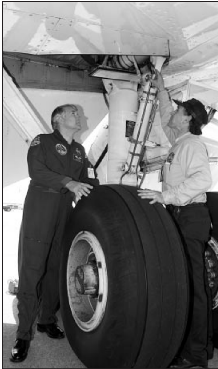
Bud Meins and Johnny LeMaster inspect the landing gear of a KC-135 as part of the preflight aircraft check. An average preflight examination for this plane takes an hour and a half.
