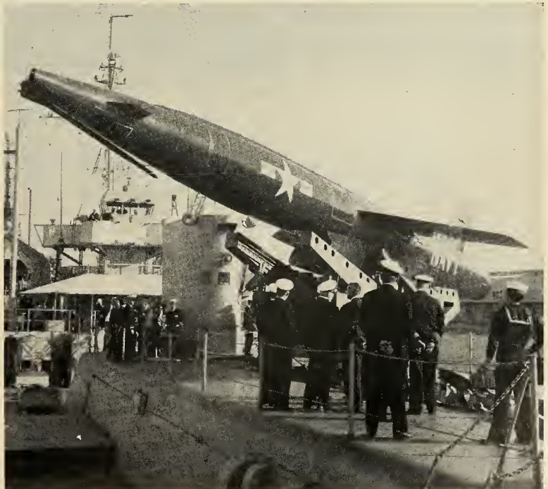
FIRST REGULUS -ARMED LST is the USS King County, an experimental vessel serving the Pacific Missile Test Range. It will test the missile launching system and will train submarine crews.
