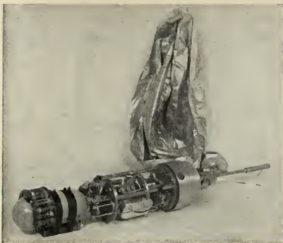
TYPICAL EXAMPLE of Purr-Kee payload. Tank in the foreground and balloon in rear are parts of recovery gear.
