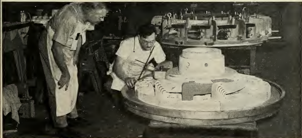
All pattern equipment is carefully checked for accuracy in the foundry pattern shop.
