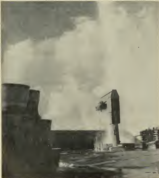
EXPLOSIVE FORMING technique, used to form unusual configurations from preformed welded tubes, speeds production.
