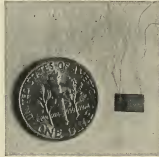
VIDEO AMPLIFIER: made with a tiny wafer from a ribbon of germanium crystal. This function block also works like a radar amplifier sub-system. Gain is essentially flat to frequencies of several megacycles.
