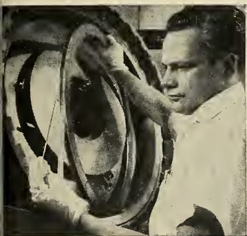
CRYSTAL GROWING techniques developed by Westinghouse have already produced germanium dendrites 300 feet long in the special furnace shown at left, above. Crystal ribbons of almost any length are possible. The take-up reel at right holds 300 feet of the brittle dendrite with each turn cushioned in glass-cloth tape.
