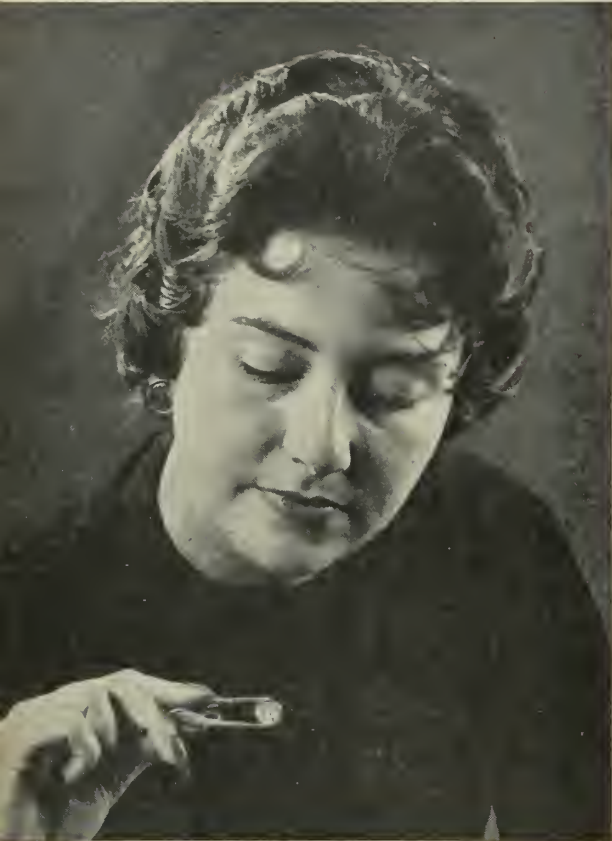
POWER AMPLIFIER: Button-sized molecular electronic device held by girl with a pair of tweezers performs the same amplifying function as a conventional 5-watt amplifier, has a frequency range from zero to 20,000 cycles. Working element is a block about as large as the head of a pin.
