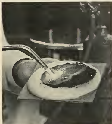
COPPER coin is melted with acetylene torch on surface of D-65. Elbert Davis, Dyna-Therm vice-president, invented it.
