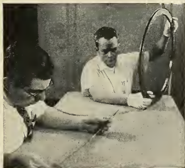
CRYSTAL GROWING techniques developed by Westinghouse have already produced germanium dendrites 300 feet long in the special furnace shown at left, above. Crystal ribbons of almost any length are possible. The take-up reel at right holds 300 feet of the brittle dendrite with each turn cushioned in glass-cloth tape.
