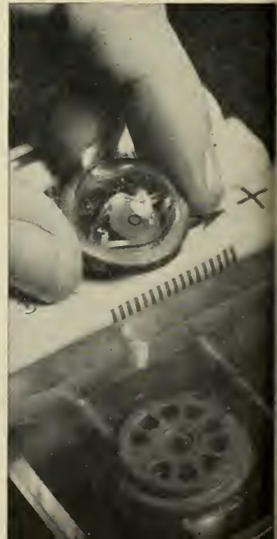
LIGHT TELEMETRY SUB-SYSTEM: a single light-responsive monolithic element delivers output whose frequency is a measure of light intensity.
