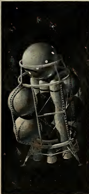
OUTERSPACE VEHICLES —Sundstrand has been the prominent factor in the development of a solar mechanical engine which, using an advanced working fluid, is capable of providing a continuous source of power generation for satellites, platforms and other space vehicles. A closed cycle power conversion system, this exotic, advanced power system is typical of the research and development work currently being conducted by Sundstrand for outerspace vehicles.
