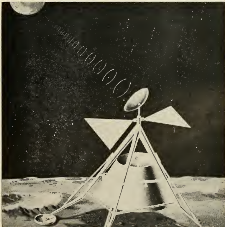
PROJECT SURVEYOR spacecraft, powered by a Centaur launch vehicle, would make a soft landing on the moon carrying a payload of some 200 lbs. of instruments.
