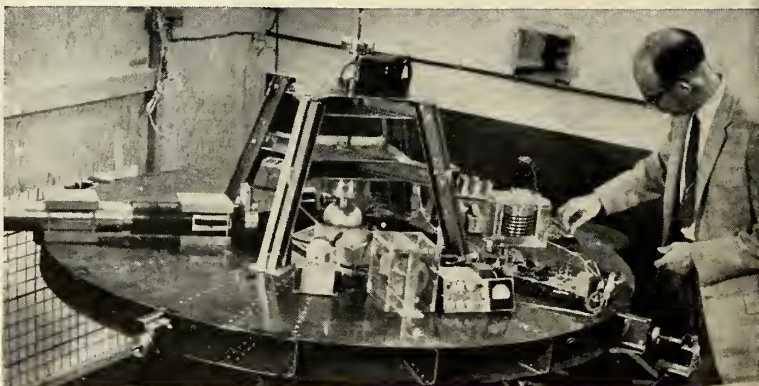
SATELLITE ENVIRONMENT is closely approximated in this circular table, balanced on a metal sphere supported on a cushion of compressed air, at NASA's Ames facility.
