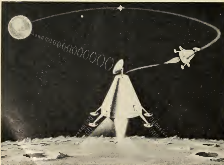
PROJECT PROSPECTOR unmanned spacecraft will be boosted by the Saturn vehicle to a soft landing on the moon, where it will explore by remote control.
