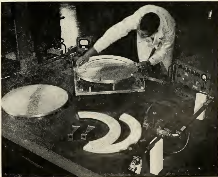
RADOMES THAT provide radar antennas with protection against the elements must be highly transparent to radar waves. Here, a Stanford Research Institute engineer determines electrical characteristics of new high-strength radome walls. The equipment shown permits the use of a narrow strip of the radome to simulate a large, flat radome panel.
