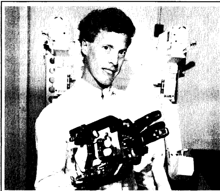
Top: Tom Grubbs, Crew and Thermal Systems Division mechanical engineer, checks the redesigned robot hand destined for EVA Retriever's Phase 2 Demonstration in January 1989. Grubbs designed the hand now on the Retriever's right arm, and this update adds touch and pressure sensors. Left: Lockheed consultant Dr. John Jameson works with the remote manipulator hand he designed as an alternative to spacesuit gloves. A robotic derivation of the design, now being fabricated by JSC's Technical Services Division, will be placed on EVA Retriever's left arm for the January 1989 demonstration. Far left: Electrical engineers Larry Li, left, and Cliff Hess study a variety of the hands under development for EVA Retriever.
