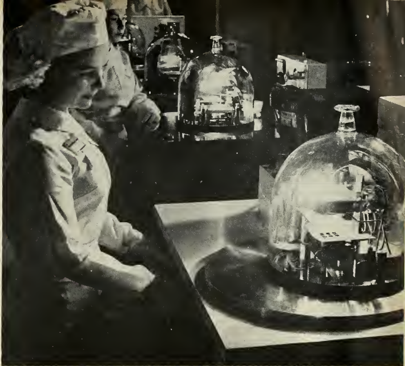
EVAPORATION PRODUCTION techniques yield pairs of gold and aluminum stripes on a 0.025-in.-square germanium wafer for mesa transistors at Motorola's Semiconductor Products Division in Phoenix. When the wafer is cut, each pair of stripes will become one transistor.
