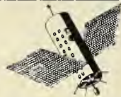
Orbiting Geophysical Observatory —1000 lb. geophysical research satellite designed for a near earth circular polar orbit or an inclined highly elliptical orbit.
