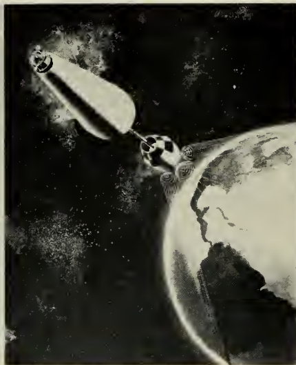
LEFT —Satellite power supply, SNAP 10 (0.3 KW), available in two years. CENTER —SNAP 2 (3 KW) and SNAP 8 (35 KW) units available 1963-5 for 24-hour communications satellite. RIGHT —Nuclear system (1967) to power electrically-propelled vehicle.
