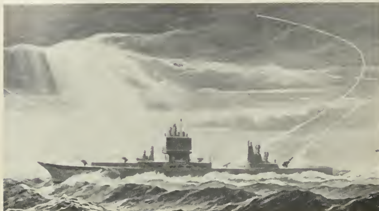
MISSILE CRUISER queen, the nuclear-powered Long Beach, carries (stern to bow) Taloses , Polarises , Asrocs and Terriers in this graphic artist's conception.
