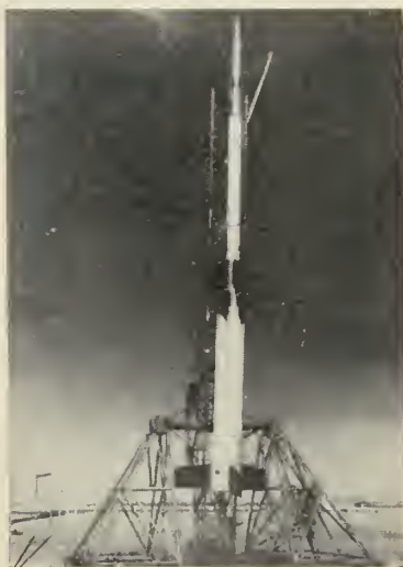
AUSTRALIAN-built Long Tom rocket on launcher at Woomera. It is 27 feet long and weighs nearly one ton.
