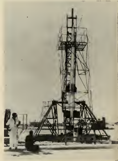
ANOTHER two-stager, also Australian-built and used at Woomera, is the 21-ft.-long Aeolus, weighing a half-ton.
