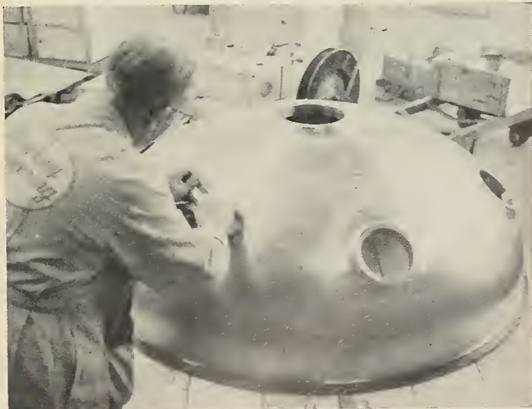
THOUGH the wall thickness of this forward bulkhead for a large solid-propellant rocket motor gets as low as .070 in., thickened sections boost the total weight.
