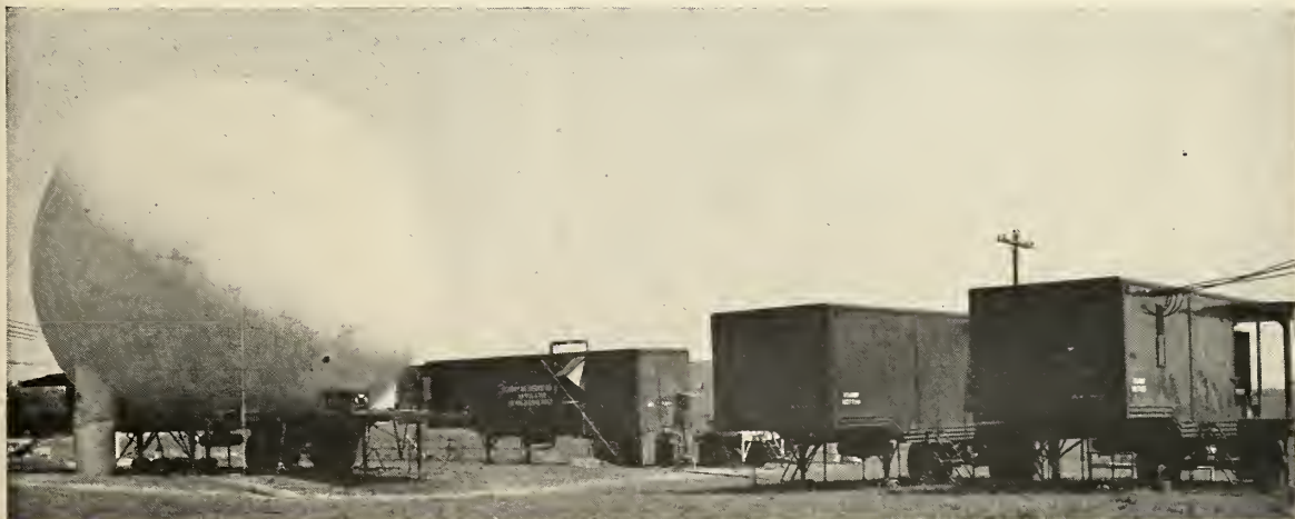
FRESCANAR SYSTEM set up and ready for operation. At left is the plastic radome housing 15-ton antenna which obtains information and sends it to radar van on its right. Only physical connection between radar van and antenna is waveguide for transmission of the microwave energy. Two units on right are active and standby diesel generator vans.
