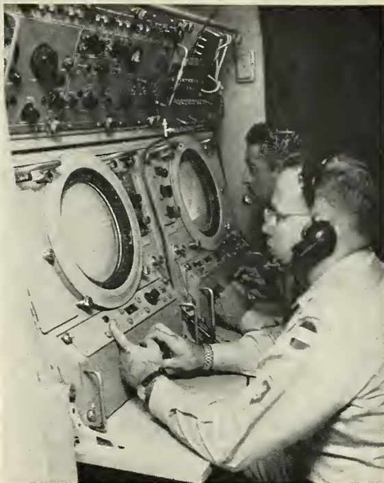
OPERATORS' POSITIONS. Scope on left shows target range and bearing; that on right, altitude. Date is transmitted instantaneously to missile batteries.
